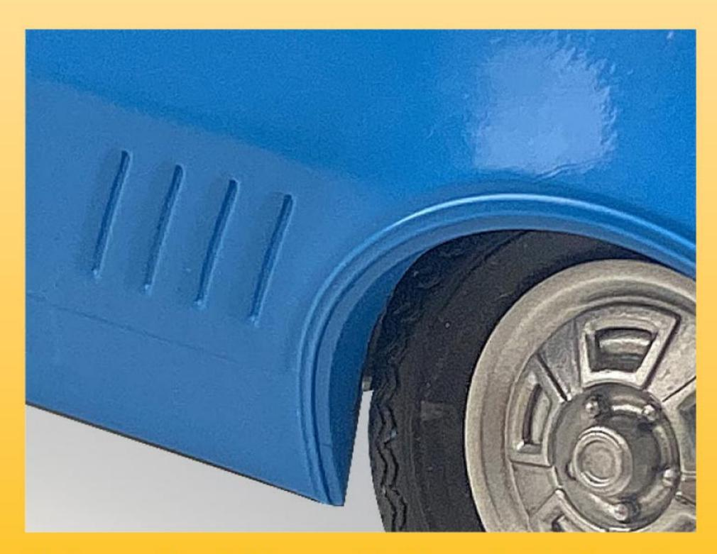
Only on the GTS model, four distinctive fins on the front quarter panels cooled the brakes.
