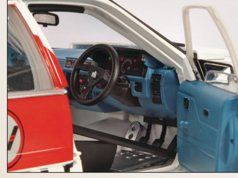
The race car interior features extra gauges, rollcage, SAAS steering wheel and seat.
