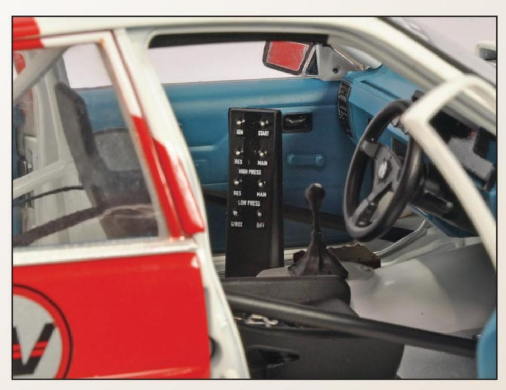
The sparse race car interior includes a switch tower. Note the arm rests are removed from the doors.
